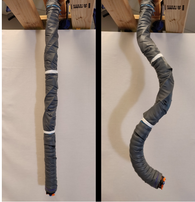
Figure 2.1: Left: A multisection continuum arm at rest, Middle: A multisection continuum arm shown actuated
